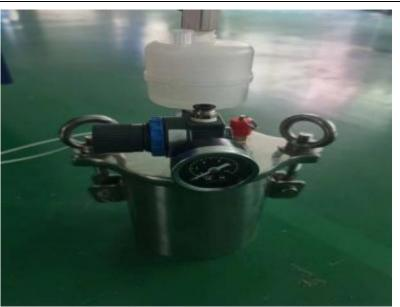
■ Flux is stocked by PP plastic pressure tank, make sure pressure stable without influenced of amount of flux.
